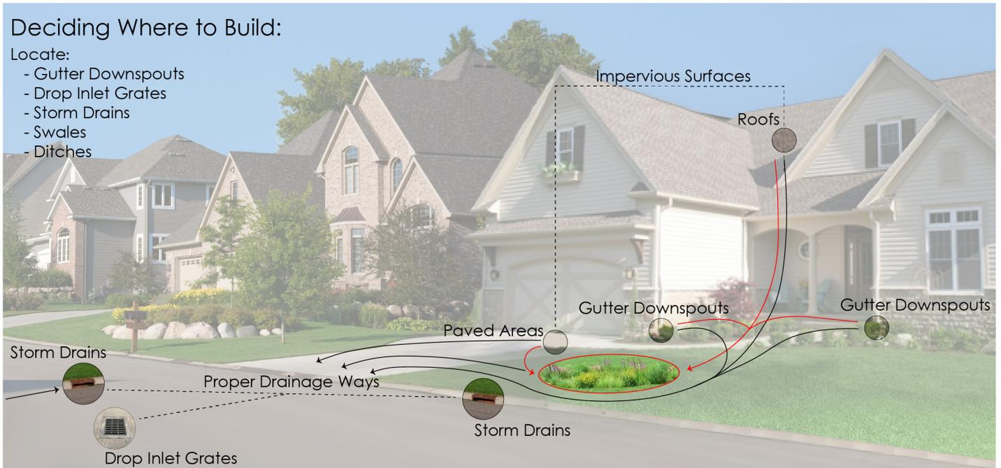
Figure 3: When determining where to build, consider the typical drainage patterns of your area, signified by the black lines above. If placed correctly, the runoff from your building will enter the rain garden system, depicted by the red lines.
