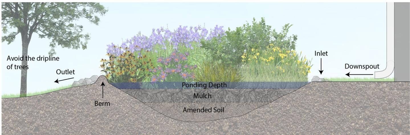
Figure 5: The layout of a rain garden should include both an inlet for runoff to enter the system and an outlet for water to exit. To protect against soil runoff, place a small berm prior to the outlet. The depression of the rain garden should be composed of amended soil and then a top layer of mulch.
